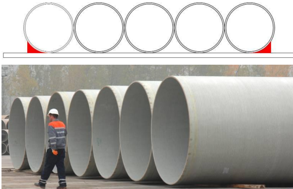
Figure 4: Storage of pipes as a single level
